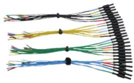
No need to pierce insulation or back-pin connectors. Fully shrouded and insulated for safety. These breakout leads simply connect into the existing cable loom and enable voltage readings to be taken from numerous sensors in the engine compartment
