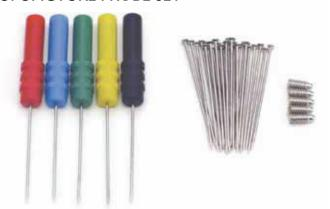
The acupuncture probes slide under the insulation of multi-plug terminals from behind the plug, allowing you to pick up signals without stripping wires or disconnecting plugs. This technique is sometimes called back-pinning. Each probe fits onto the 4-mm plug of a TA000 or similar test lead. A storage box containing spare pins and screws is included.
