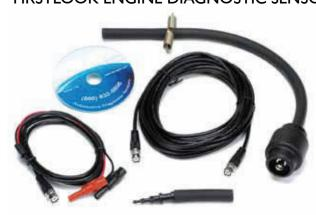
The FirstLook pressure sensor detects pressure and vacuum pulses in the inlet manifold and the exhaust tailpipe. When viewed on the PicoScope display, these pulses can give valuable diagnostic information. Can also be used with the TAO40 ACE Misfire Detective software to automatically identify misfires
