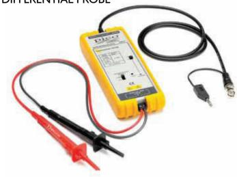
The active differential probe lets you measure floating voltages on electric motors and generators. These probes have a bandwidth of 25 MHz, with differential voltage ranges of 700V or 1400V.
