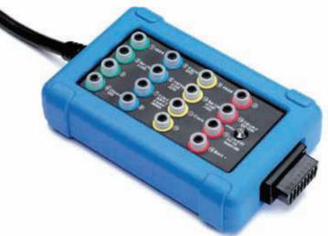
The CAN Test Box allows you to connect your PicoScope oscilloscope, or any other compatible scope, to the 16 pin diagnostic connector enabling you to monitor any signals present, such as the CAN High and Low signals. The CAN Test Box terminal pin ports are accessible with standard 4 mm plugs.
