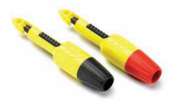
When there is no other way to get to a wire, clamp one of these on and a sharp pin pierces the insulation. Accepts 4mm plugs. Sold as a pair (1 red, 1 black)
